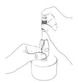
Place the impact device against the object to be measured. Then press the release button on top of the impact device with finger of right hand. The measuring value will display on LCD.
