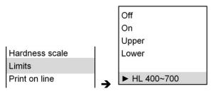
Select "On" to enable pre-set Upper/Lower Limit, and display " $\mathbf{I}$ " in Measure screen. After enabling, the Voice Prompt is enabled by default. After overrun, prompt three sounds. If the measurement is above the Upper Limit, " $\triangle$ " displays next to the readings. If the measurement is under the Lower Limit, " $\nabla$ " displays next to the readings. Select "Off" to disable Upper/Lower Limit prompt. Select "Upper" or "Lower" to adjust.
