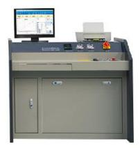
Oil source: offer high-pressure oil to hydraulic system, driving device for adding the load to specimen through the load frame. The oil source is inside of the Control cabinet.
